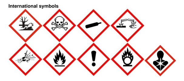
All products with such symbols should have a data sheet which can be provided by the manufacturer. These will provide all appropriate information to deal with accidents, over exposure and so on.
